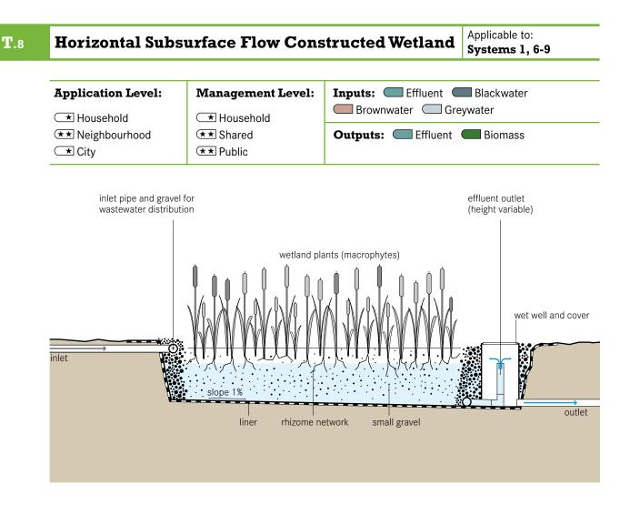
A horizontal subsurface flow constructed wetland is a large gravel and sand-filled basin that is planted with wetland vegetation. As wastewater flows horizontally through the basin, the filter material filters out particles and microorganisms degrade the organics.
